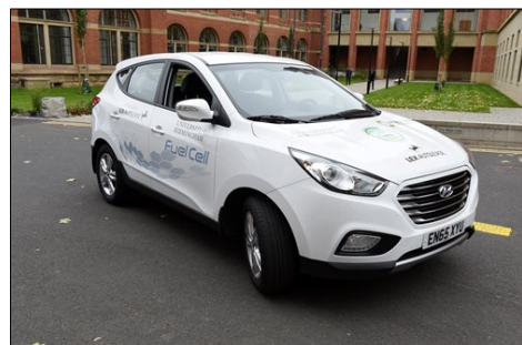
Fig.2: The University's Hyundai ix35 Fuel Cell. The vehicle is pollution free, virtually silent in operation, and is reputed to achieve speeds of 50mph and travel up to 369 miles on a full tank.
